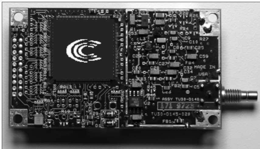
Figure 2. The Conexant Jupiter GPS Receiver (-211) With Right Angle SMB RF Connector (Bottom View -- Shown Approximately 1.5x Actual Size)
